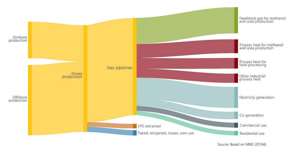
Figure 6: Flows of natural gas in New Zealand.<sup>1</sup>
