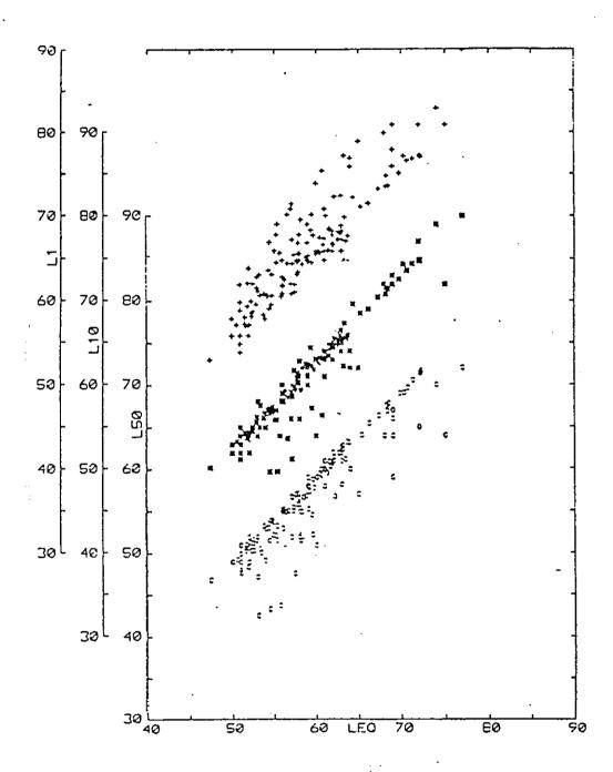
Hourly Measured Sound Level (Ln) vs Equivalent Sound Levels (Leq)
