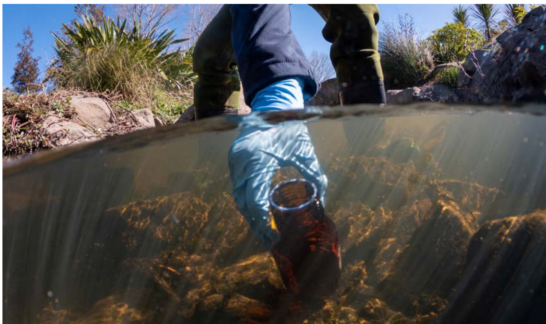
Figure 5.4: Water ecologist collecting a water sample that will be sent to a lab where technicians will extract DNA and identify traces of any species that were present in the environment.
