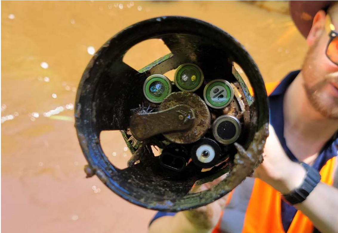
Figure 5.1: Macrophytes, biofouling, mud snails and burial of high-frequency (continuous) water quality monitoring sensors are common issues that need continuous management.
