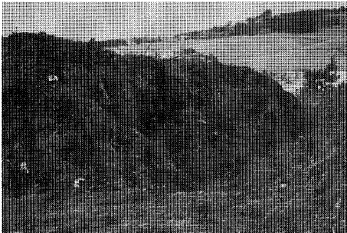
Composting windrows: turned every 10 to 14 days by front-end loader; composting period in windrows three to four months.
