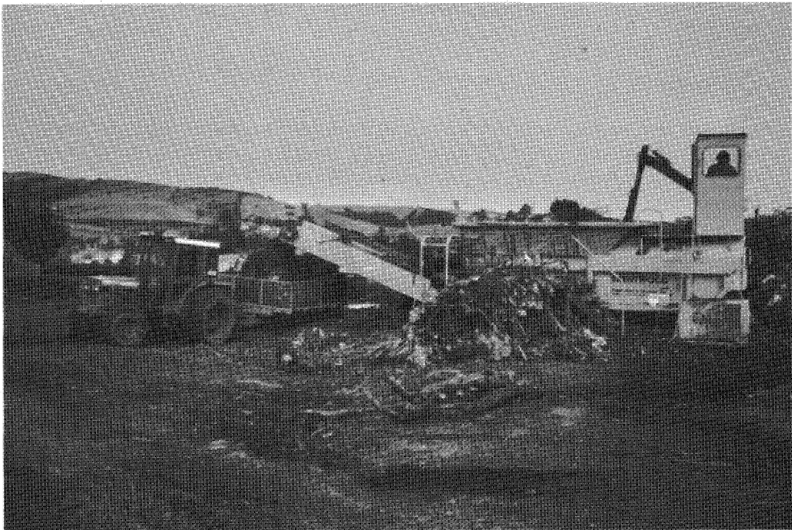
Shredding of greenwaste into trailer, which is taken to build windows. Shredder is electric, low speed and high torque.
